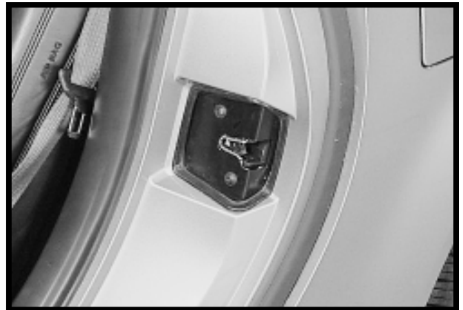
Figure 4-2, Door Latch in Body
