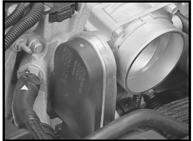
Figure 2-5, Throttle Actuator Control (TAC) Throttle Body
