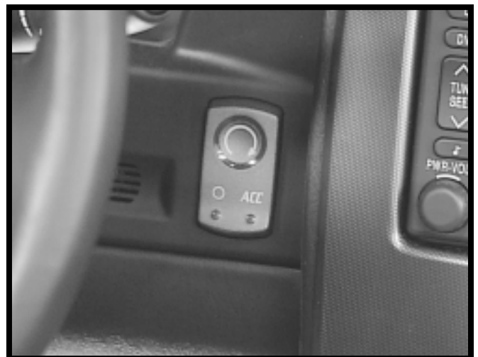
Figure 5-2, XLR Ignition Rocker Switch
