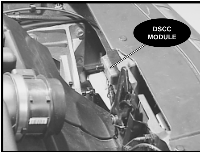
Figure 5-6, Distance Sensing Cruise Control (DSCC) Module
