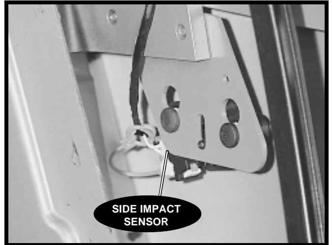
Figure 5-24, Side Impact Sensor
