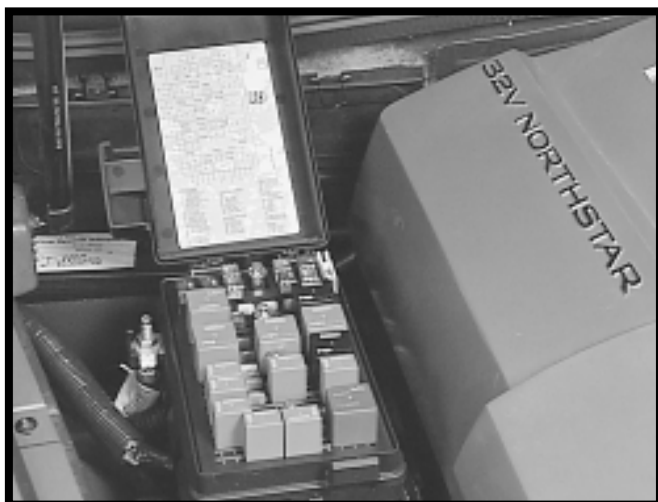
Figure 3-24, Underhood Bussed Electrical Center (UBEC)
