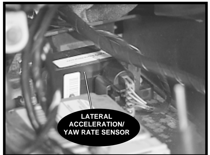
Figure 4-5, Lateral Acceleration/Yaw Rate Sensor
