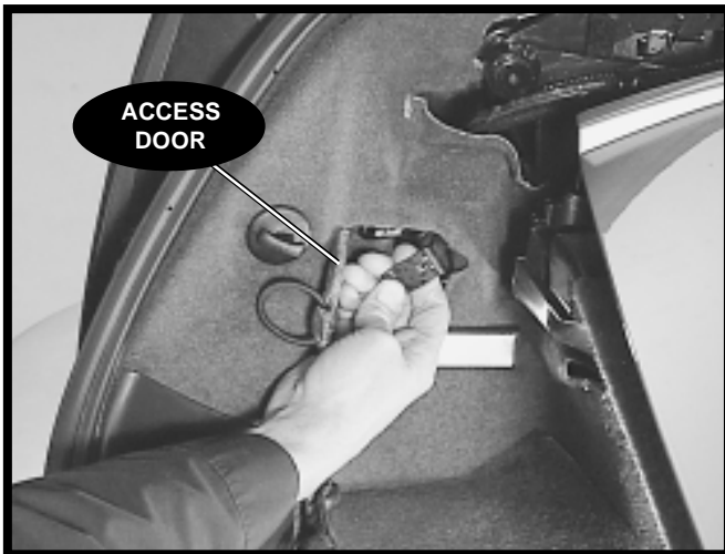
Figure 3-10, Manual Door Release Handle in Trunk
